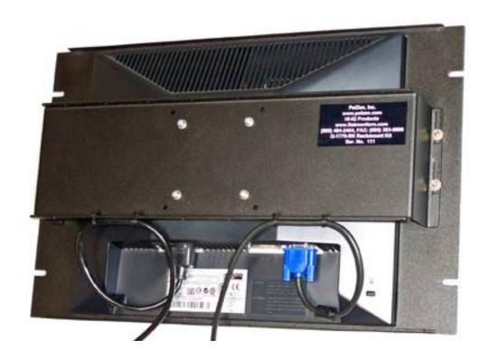
7. The monitor is now assembled. Before mounting it onto a rack, test the rackmount monitor assembly by connecting it to a computer. When done, mount the assembly onto a rack with the four black 10-32 rackmount screws provided.
