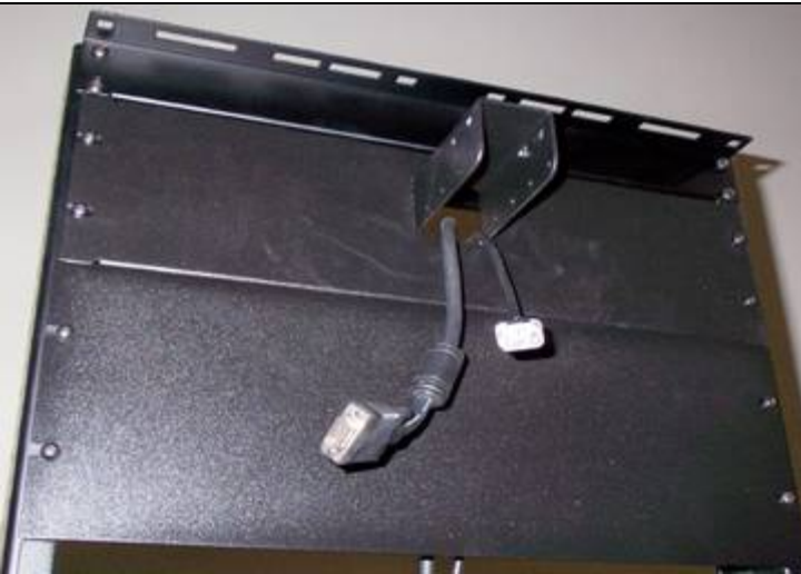
Figure 9. Cables are fed through the cable-entry hole.
