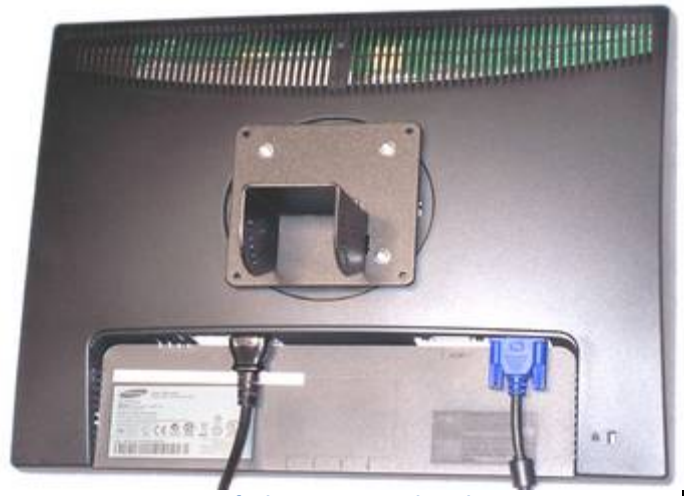
Figure 8. Rear view of adapter mounted on the monitor.
