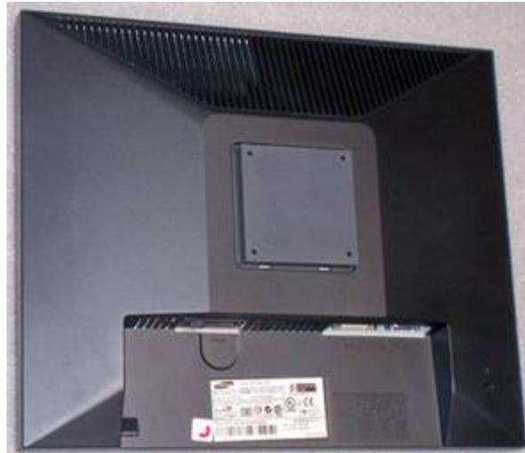
4. Mount the U-bracket onto the monitor with a 4 mm X 25 mm metric screw, a No. 8 lock washer and a No. 8 flat washer into each one of the four VESA mounting holes.
