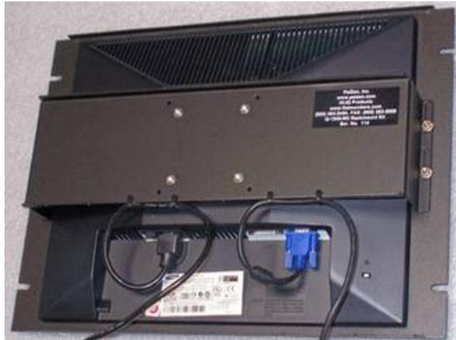
8. Use tie wraps to secure the cables onto the holes on the lower flange of the U-Bracket. Then trim all excess lengths of the tie wraps with a wire cutter.
